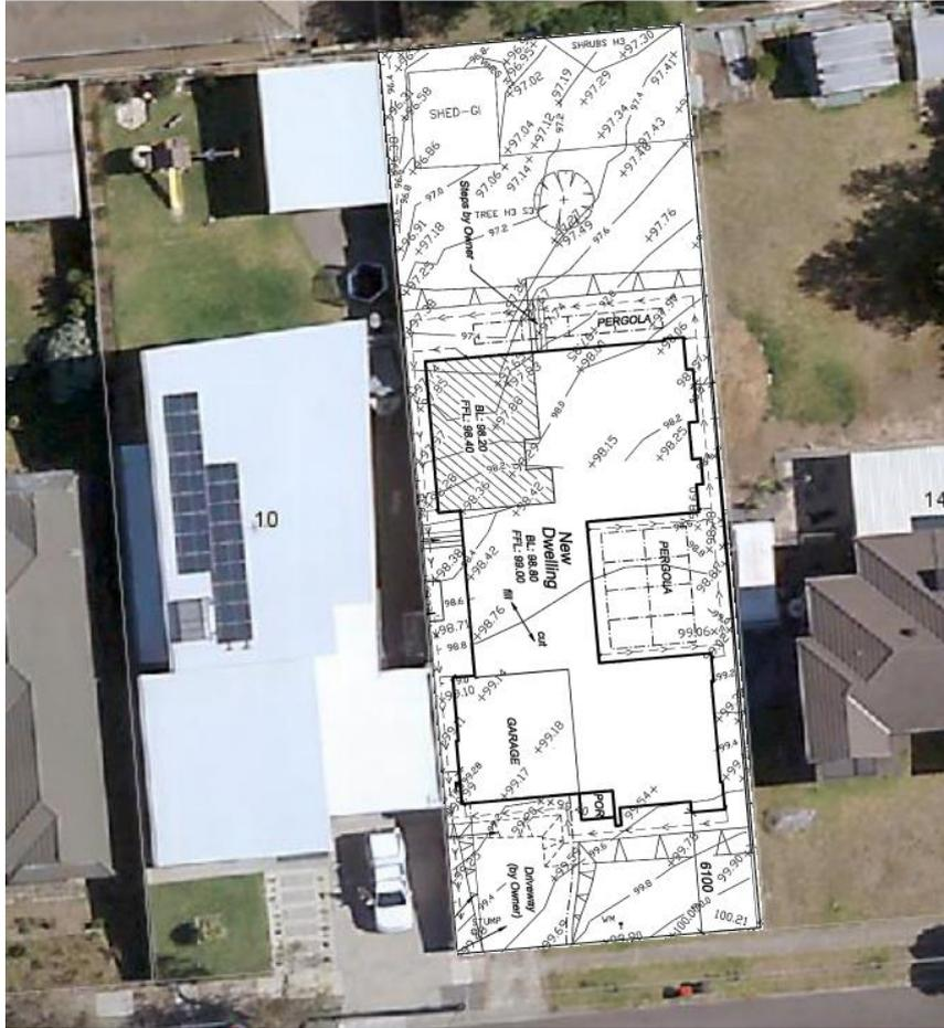
**Figure 1:** Site plan of dwelling superimpose on aerial image.
